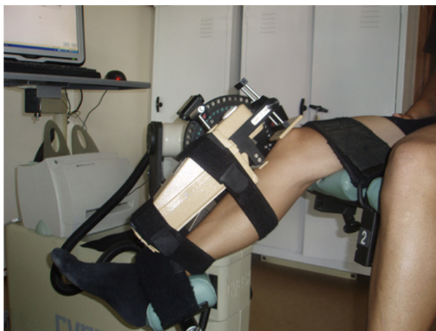
Fig 2. The experimental setup with the right knee joint centered on the axis of rotation of the dynamometer and the KT-2000 securely attached to the participant's tibia.
